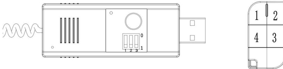
1. The external decoding module uses the standard HCS301 format open code, the frequency 433MHZ/868MHZ is optional,
