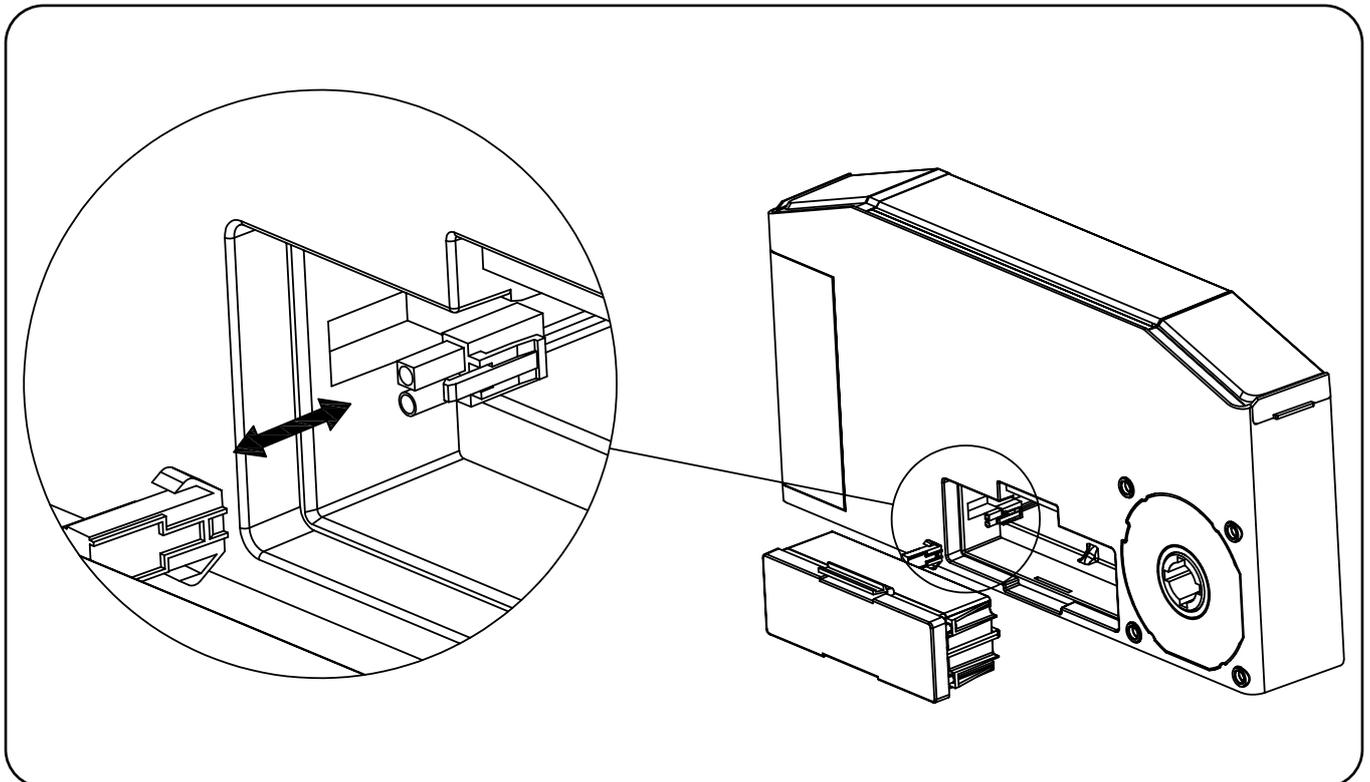
Step 2: Connect the battery and put it into the card slot.
