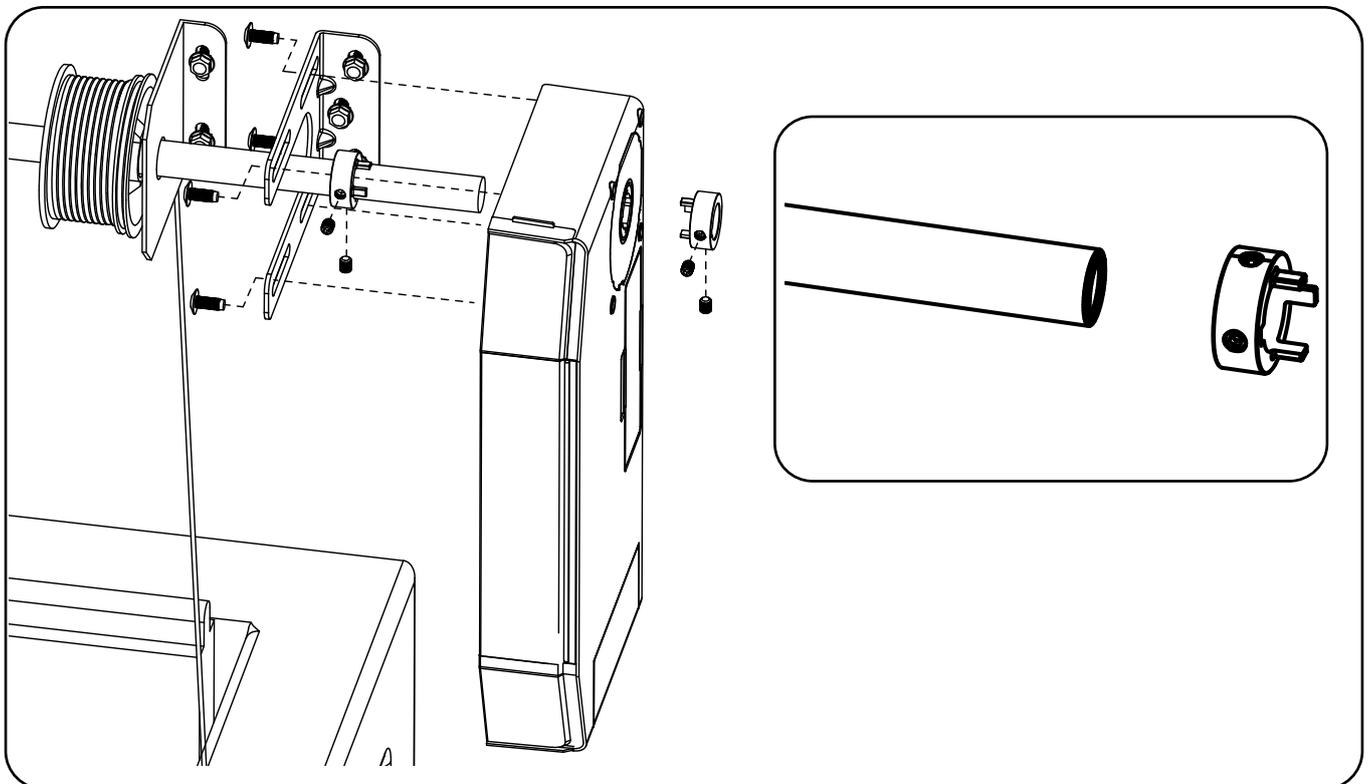
Step 3: Insert the first positioning ring then install the Multi-Drive. Use M8\*10mm set screws to lock the positioning ring.
