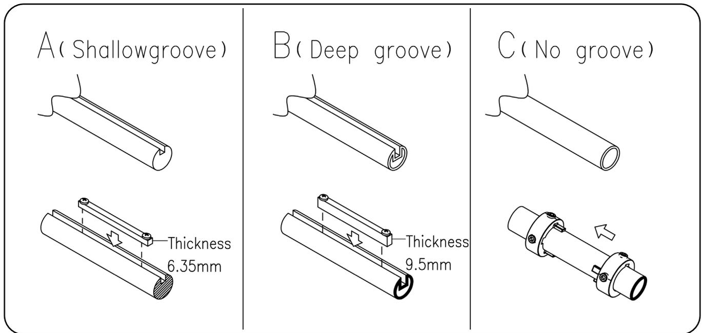
4.3 Steps for installing with door central axis types A and B (same method) are as follows:
