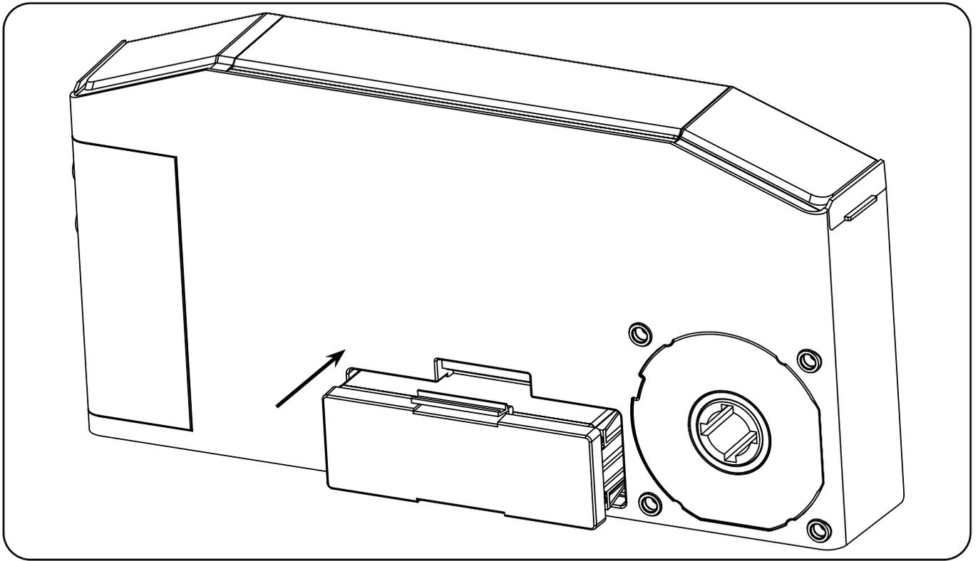
Step 3: Insert the battery module and the installation is complete.
