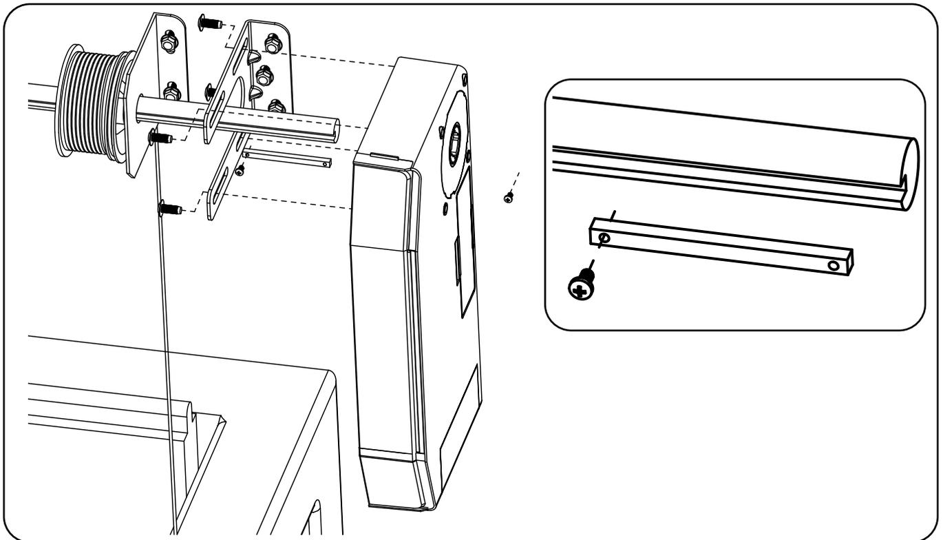
Step 3: Install the motor and rotate the central shaft to install keyway pin.
