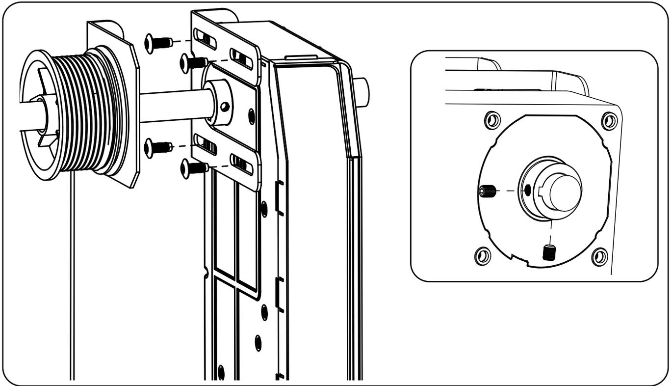
Step 4: Use M8\*16mm bolts to fix the bracket and the motor. Insert the second positioning ring and lock the M8\*10mm set screws.
