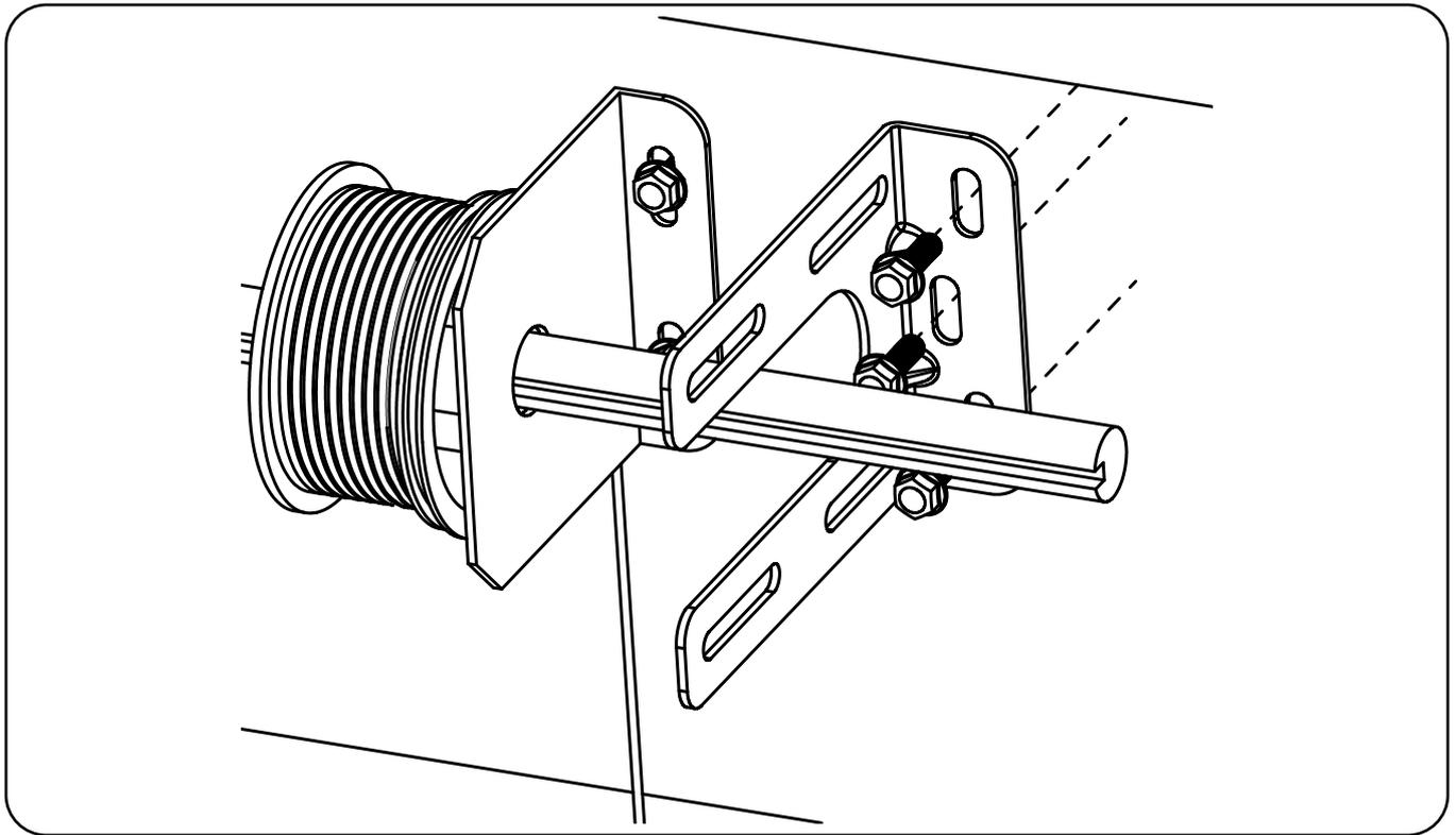
Step 2: Fix mounting bracket (180° reverse is supported).
