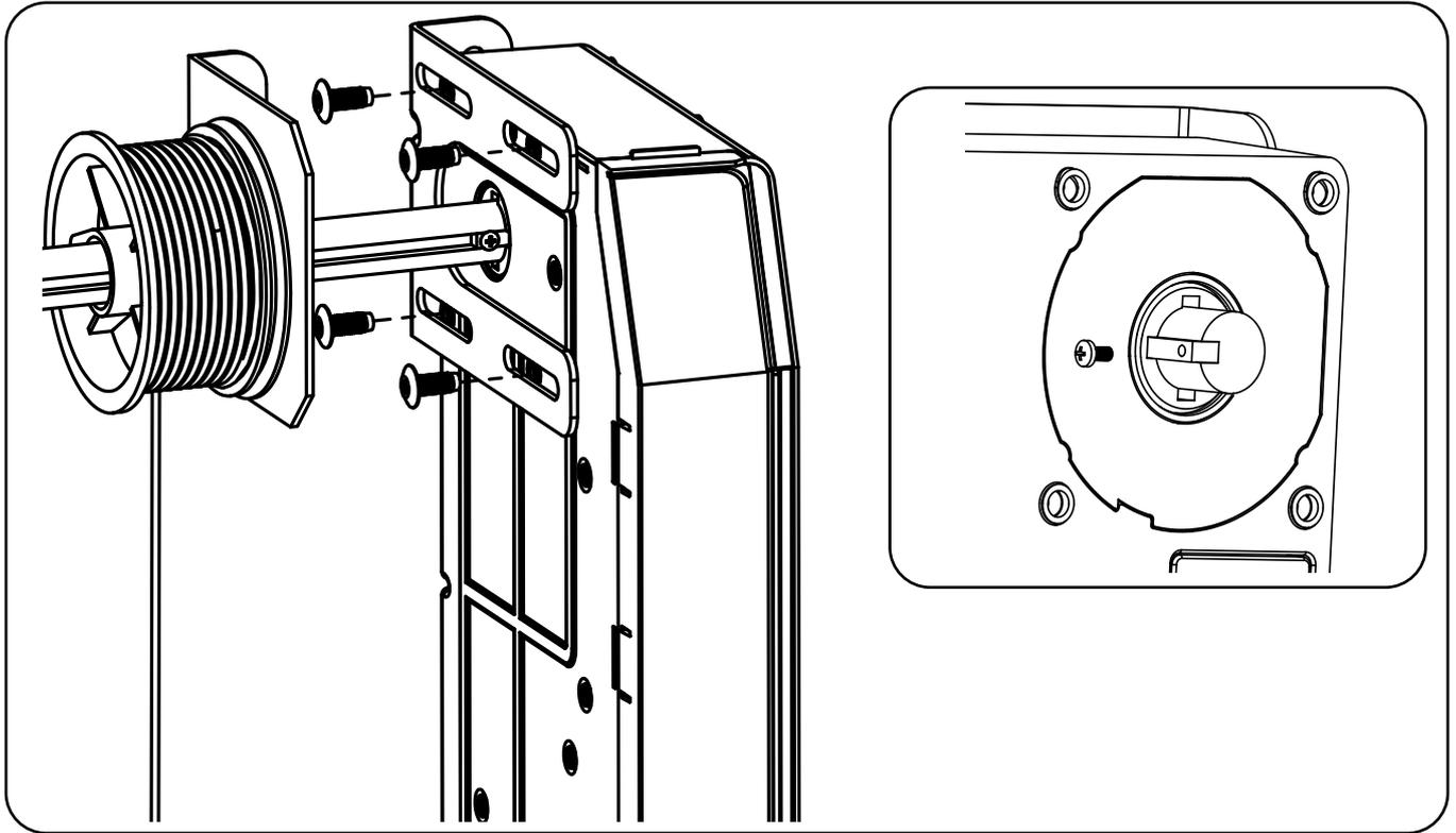
Step 4: Fix the bracket and motor with M8\*16mm bolts, and fix the keyway pin with M4\*8mm screws.
